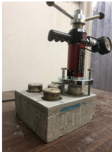
Figure 10 Pull off tests on cores
