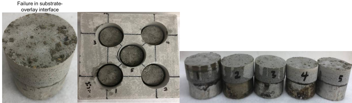
Figure 11 Neat polymer concrete overall pull off test
