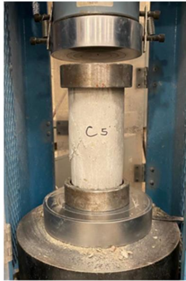
Figure 4 Compression Test Result of PolC Failed Specimen
