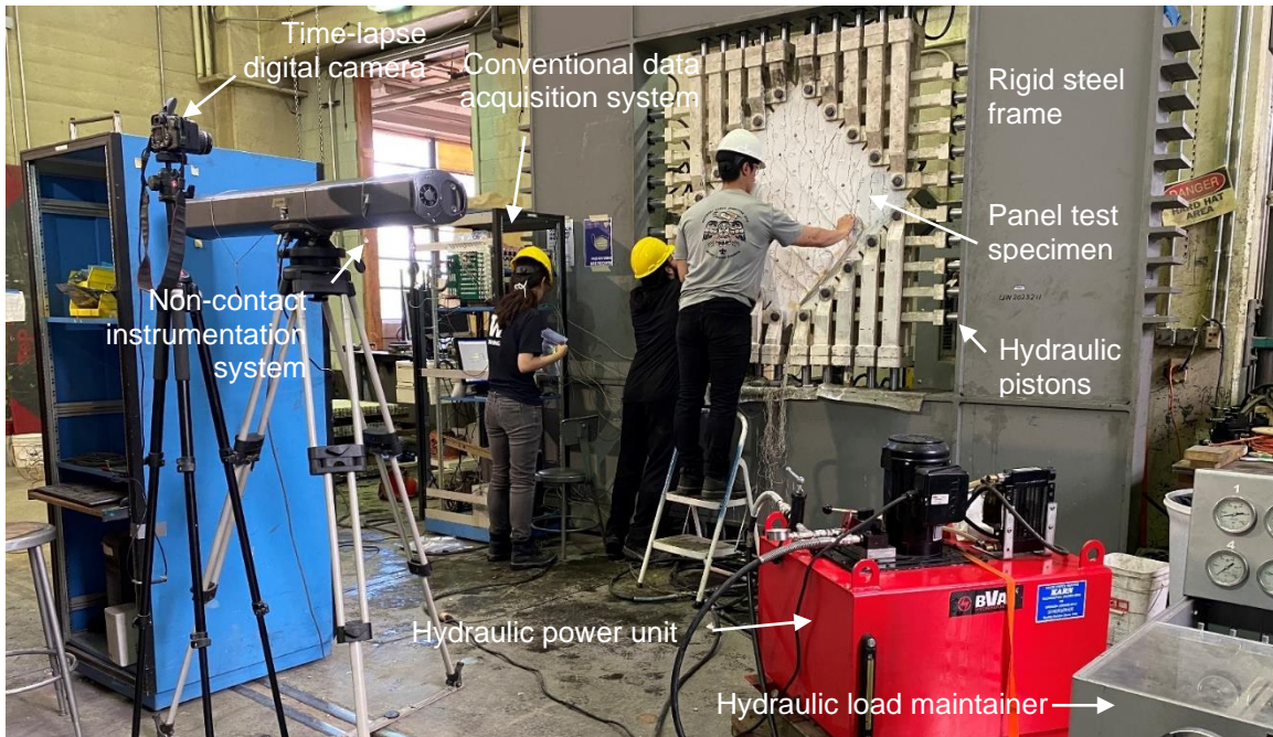
Fig.3. UW SETL Panel Element Tester setup
