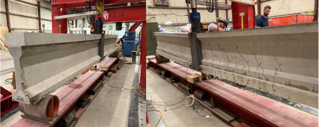
Figure 1. Continuity connection test (left) to induce positive moment in the connection and (right) to induce negative moment in the connection
