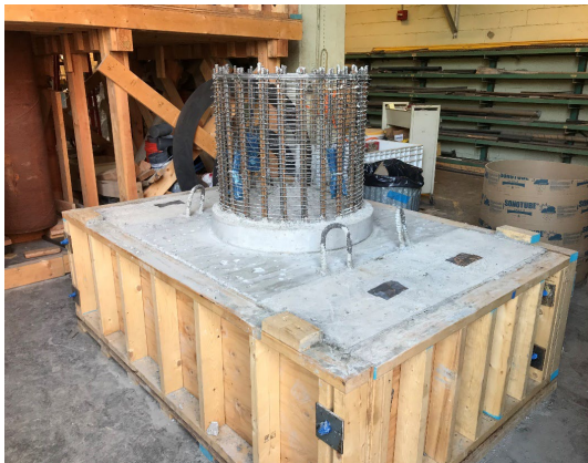
Figure 3. Photo of Shaft Reinforcement and Cast Base
