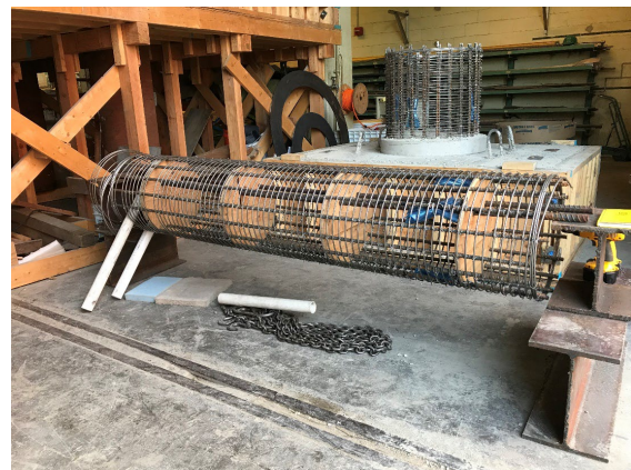
Figure 4. Photo of Column Reinforcement Cage
