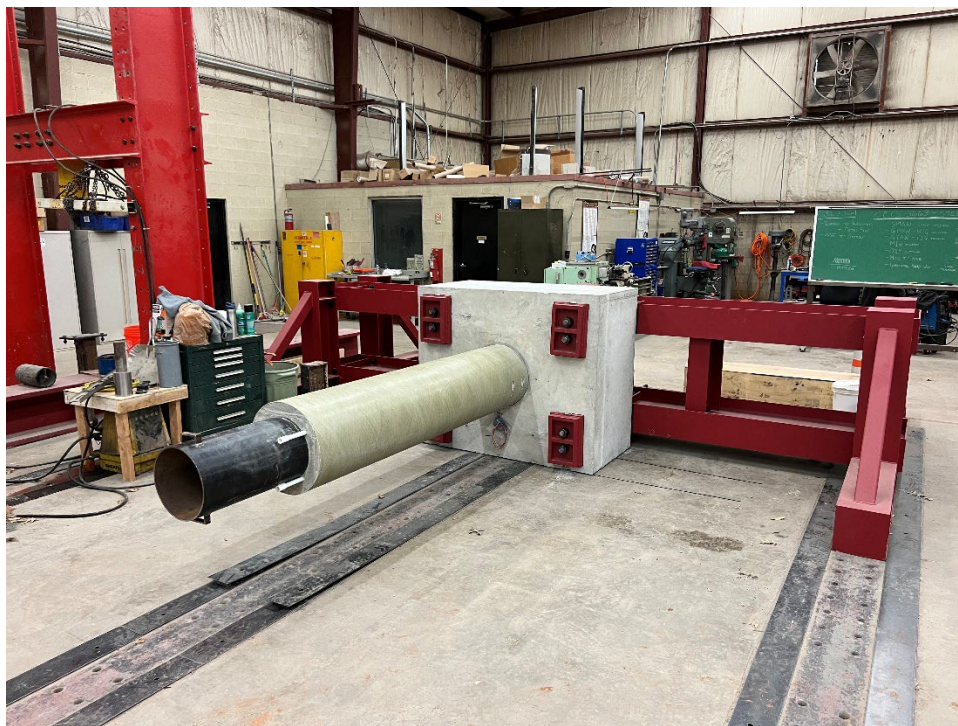
Figure 15. Completed HC-FCS Specimen Within Column Test Fixture Awaiting Installation of Loading Stub
