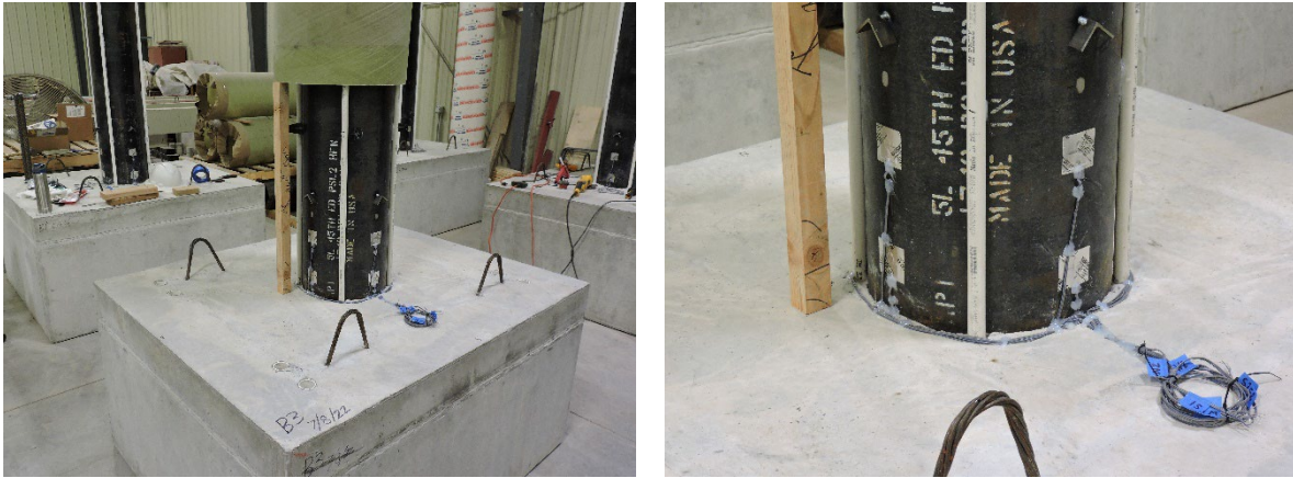
Figure 6. Strain Gage Installation for Measuring Longitudinal Stresses in the Steel Tubes
