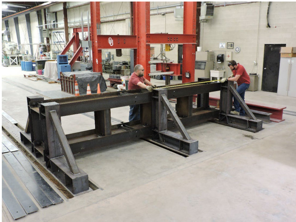
Figure 14. Completed Column Test Fixture Base Mounted to Fears Lab High Bay Strong Floor
