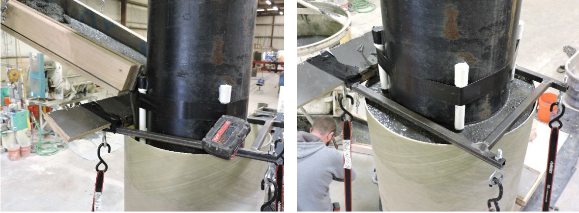
Figure 10. UHPC Inner Concrete Core Placement (l) and Completed Specimen (r)
