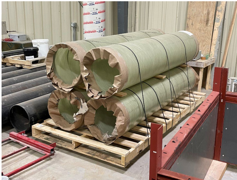
Figure 3. FRP Tubes for HC-FCS Column Test Specimens
