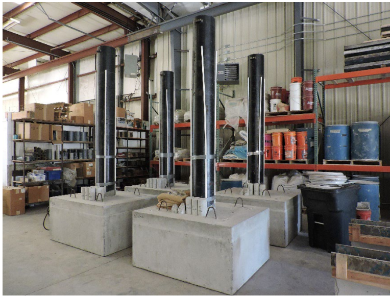
Figure 5. Completed HC-FCS Column Bases with Embedded Steel Tubes
