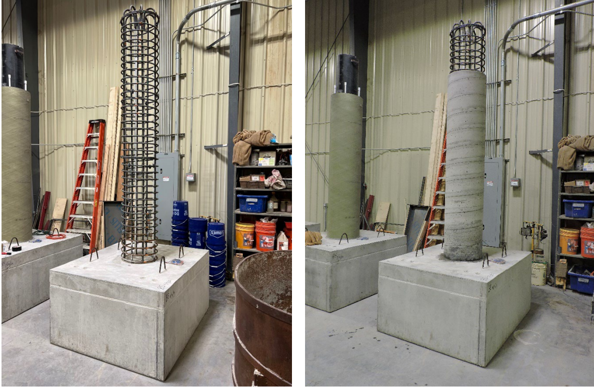
Figure 12. Conventional, Circular, Solid RC Column Reinforcing Cage (l) and Completed Specimen (r)
