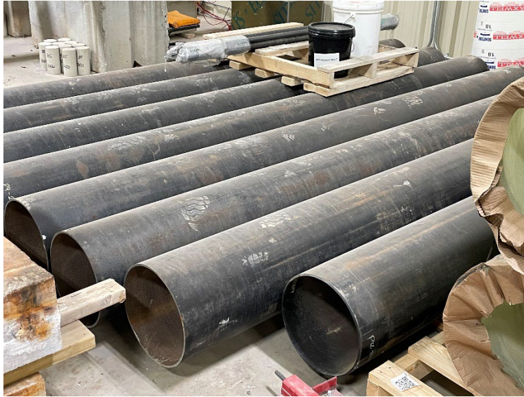
Figure 2. Steel Tubes for HC-FCS Column Test Specimens
