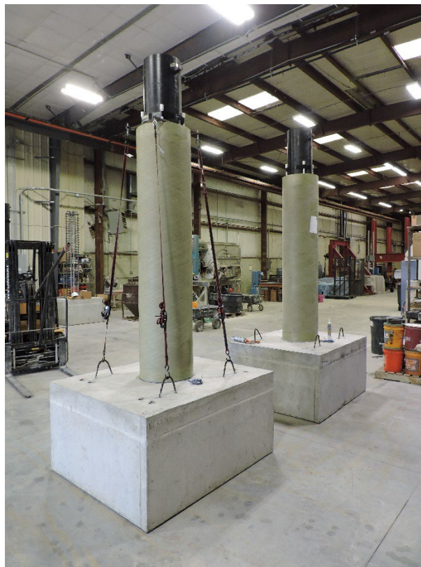
Figure 7. HC-FCS Columns Prepped for Concrete Core Placement
