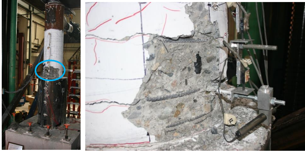
Figure 3.43. Specimen 30-21-LD Exposed Longitudinal Reinforcement at 5.5% Drift
