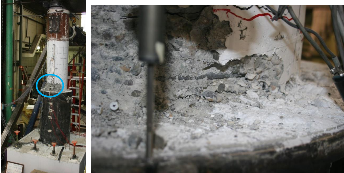
Figure 3.22. Specimen 30-21-R Exposed Transverse Reinforcement at 4.0% Drift
