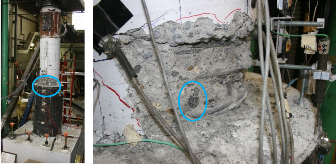
Figure 3.25. Specimen 30-21-R Exposed Northern Longitudinal Reinforcement at 5.5% Drift
