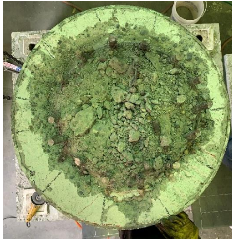
Figure 3.52. Top of Specimen 30-21-LD Pile with Column Removed
