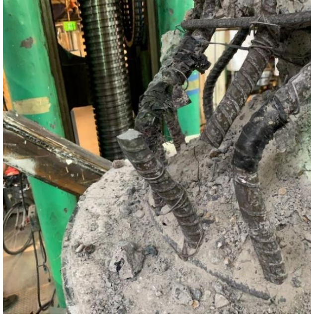
Figure 3.31. Specimen 30-21-R Fractured Longitudinal Reinforcement
