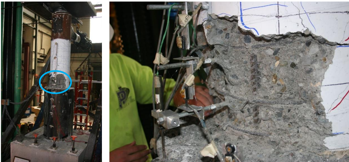
Figure 3.45. Specimen 30-21-LD Increased Spalled Region at 5.5% Drift
