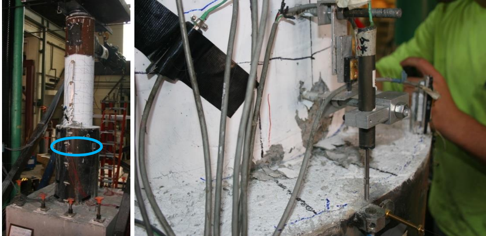
Figure 3.38. Specimen 30-21-LD 1 st Spalled Region on Northern Column Face at 2.4% Drift
