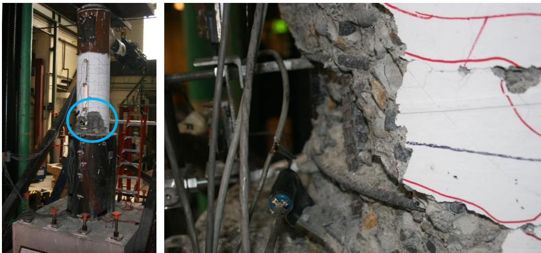
Figure 3.48. Specimen 30-21-LD Buckled Longitudinal Reinforcement on Southern Side of Concrete at 5.5% Drift
