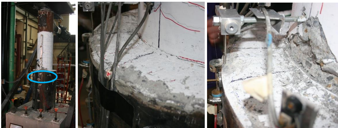
Figure 3.1. Specimen 30-21-LD a) Concrete Damage at the Edge of the Pile and b) Concrete Damage Near Base of the Column at 2.4% Drift
