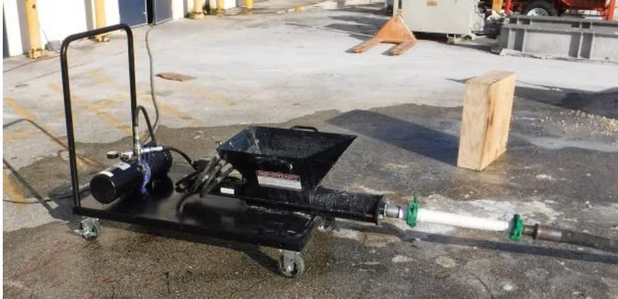
Figure 15. Black-Jack Pump, reducer and hose.
