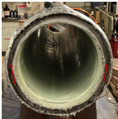
Figure 4. GFRP Slip liner using wood spacers [3]
