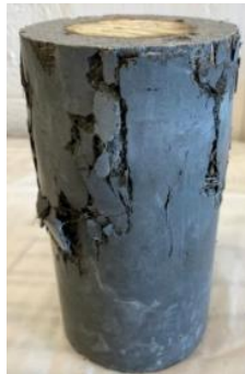
Figure 14. Failure mode of one of tested specimen.
