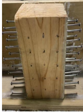
Figure 17. Timber block with 10D nails.
