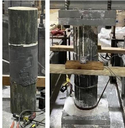
Figure 38. Large-scale specimen 10 – Max. Load: 150 kips
