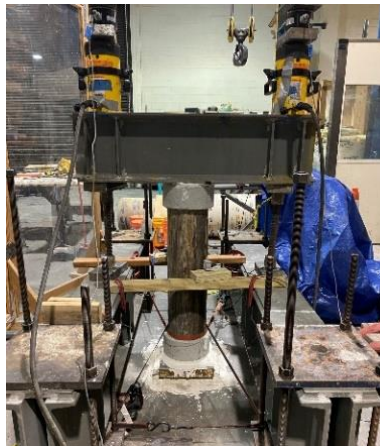
Figure 33. Large-scale specimen 04 – Max. Load: 11.0 kips
