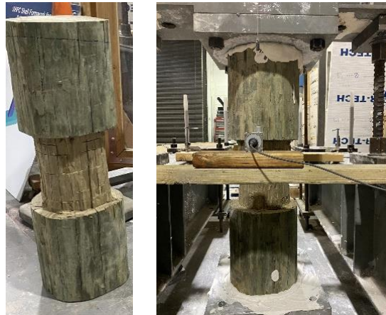
Figure 39. Large-scale specimen 11 – Max. Load: 110 kips
