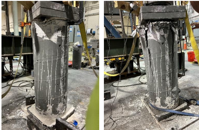
Figure 48. Large-scale specimen 20 – Max. Load: 664 kips
