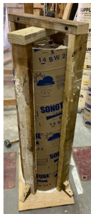
Figure 28. Construction process for complete shell encasement.
