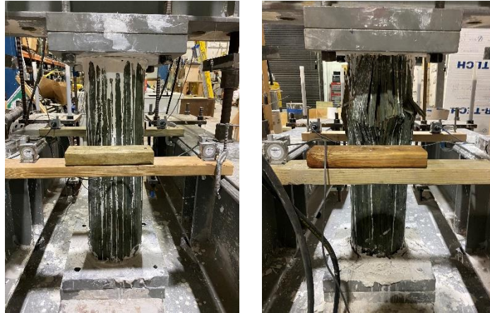
Figure 41. Large-scale specimen 13 – Max. Load: 345 kips
