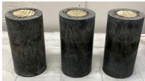
Figure 10. Sample for final timber cylinders with UHPC encasement.
