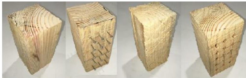
Figure 6. Different surface preparation for timber prisms
