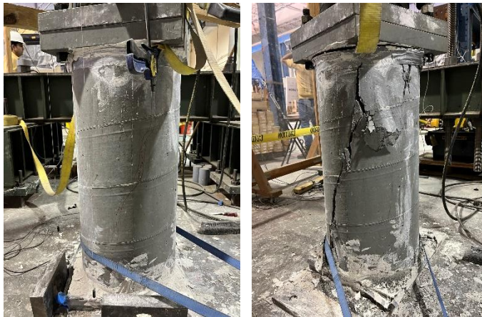
Figure 49. Large-scale specimen 21 – Max. Load: 752 kips
