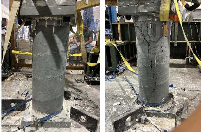
Figure 47. Large-scale specimen 19 – Max. Load: 692 kips
