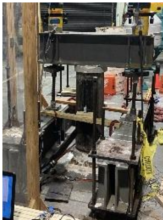
Figure 34. Large-scale specimen 05 – Max. Load: 19.0 kips
