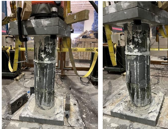
Figure 45. Large-scale specimen 17 – Max. Load: 215 kips
