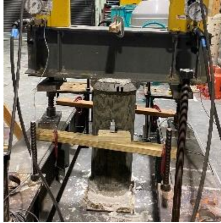
Figure 35. Large-scale specimen 07 – Max. Load: 87.0 kips
