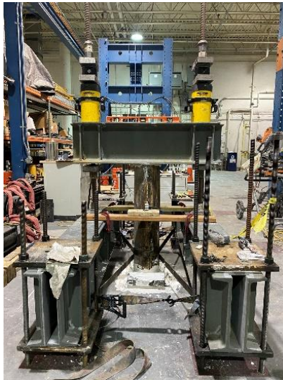
Figure 31. Large-scale specimen 02 – Max. Load: 2.5 kips
