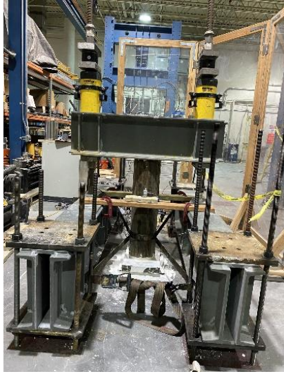
Figure 30. Large-scale specimen 01 – Max. Load: 7.7 kips
