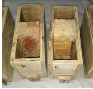
Figure 4. Formwork for pull-off specimens prior to casting UHPC.
