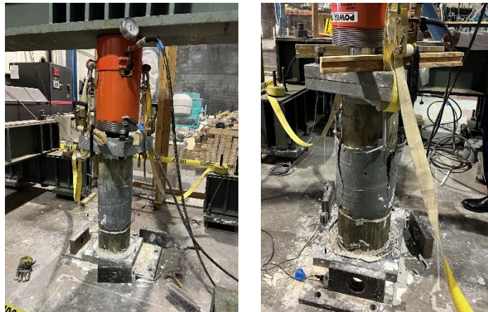
Figure 43. Large-scale specimen 15 – Max. Load: 216 kips
