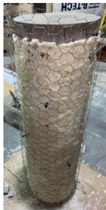
Figure 28. Construction process for complete shell encasement.
