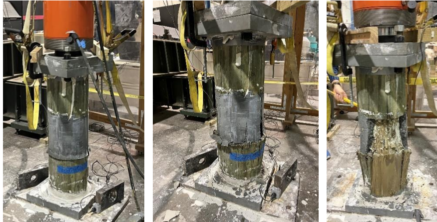
Figure 44. Large-scale specimen 16 – Max. Load: 318 kips
