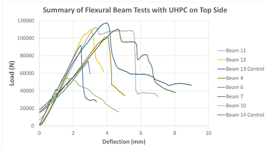
**Figure 18.** Summary of Flexural Beam tests with UHPC on Top side
