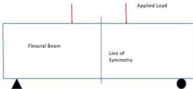
**Figure 16.** Third Point Loading Setup
