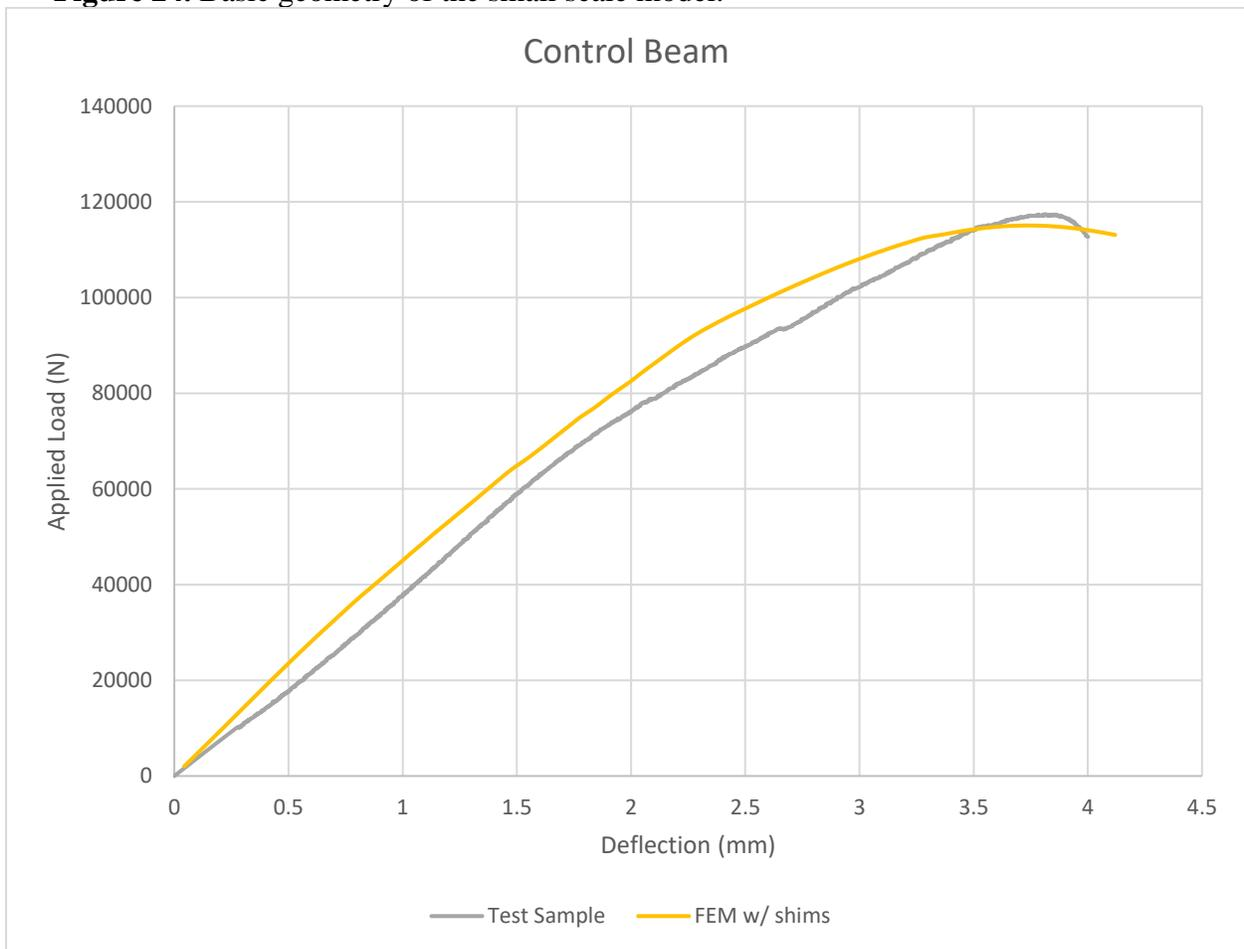
**Figure 25.** Control Beam Test results vs. FEM results.
