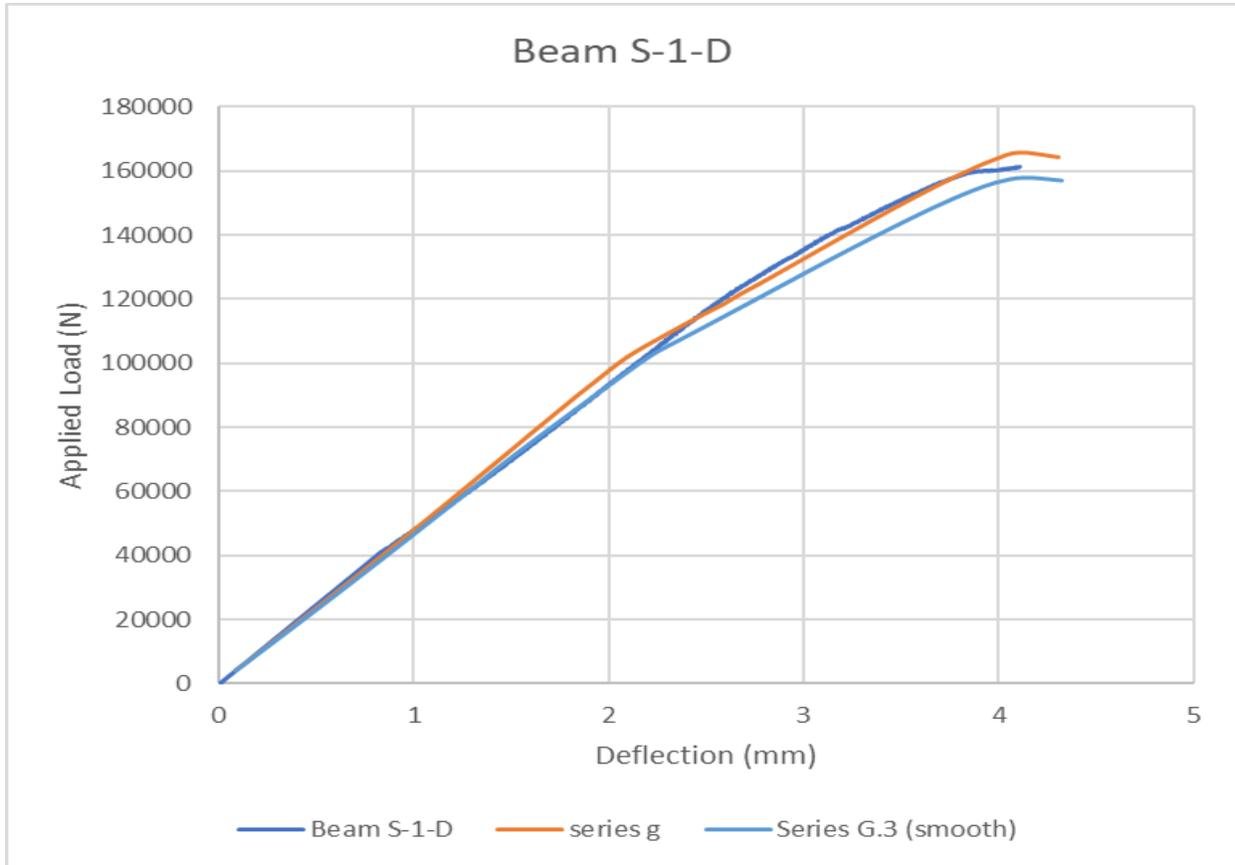
**Figure 29. FEM results for Beam S-1-D.**
