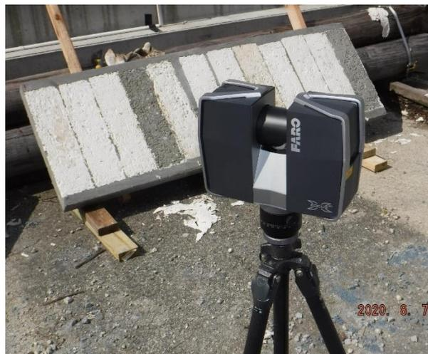
**Figure 14.** Three-Dimensional Scanner
