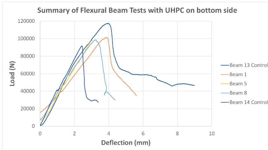
**Figure 20.** Summary of Flexural Beam tests with UHPC on Bottom side
