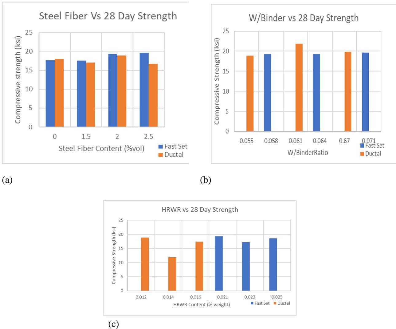
**Figure 3. Compressive Strength Test Results**
