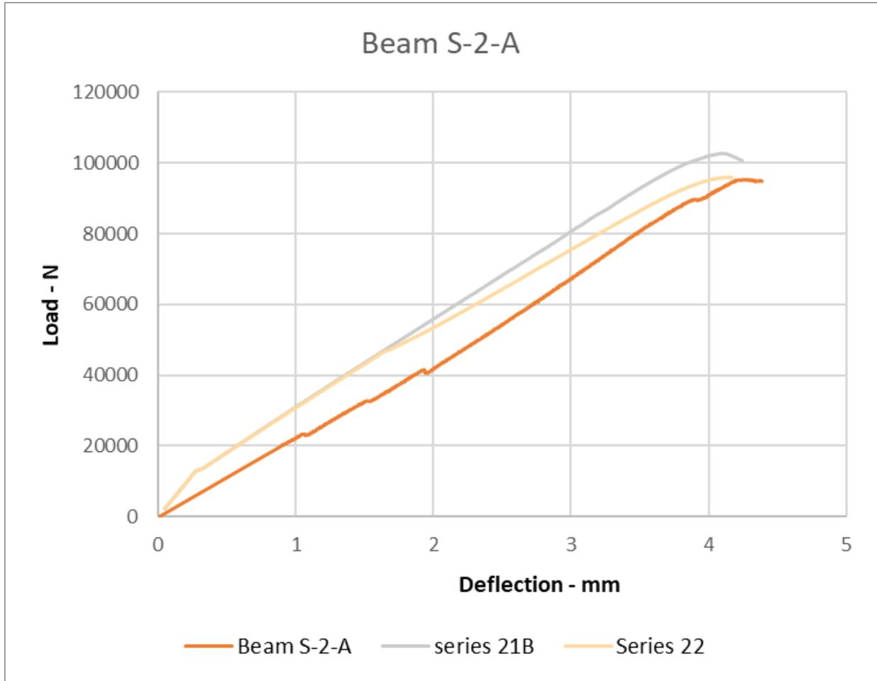
**Figure 27.** Beam S-2-A. Test results vs FEM model
