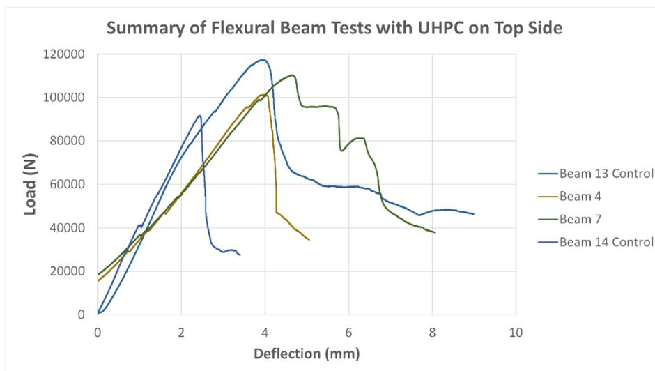
**Figure 21.** Summary of Flexural Beam tests with UHPC on Top side
