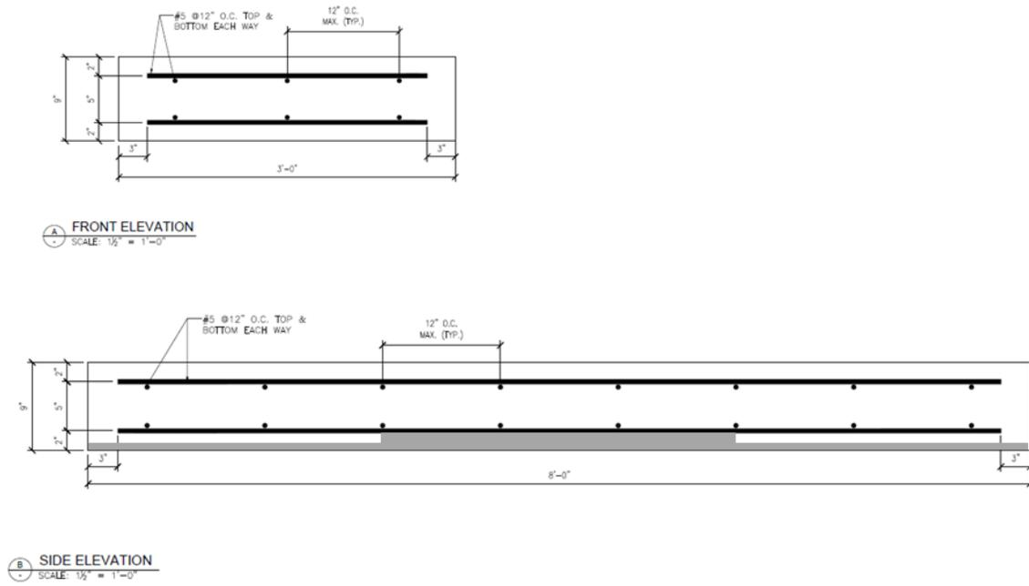
**Figure 11.** Details of the second specimen (bottom repair)
