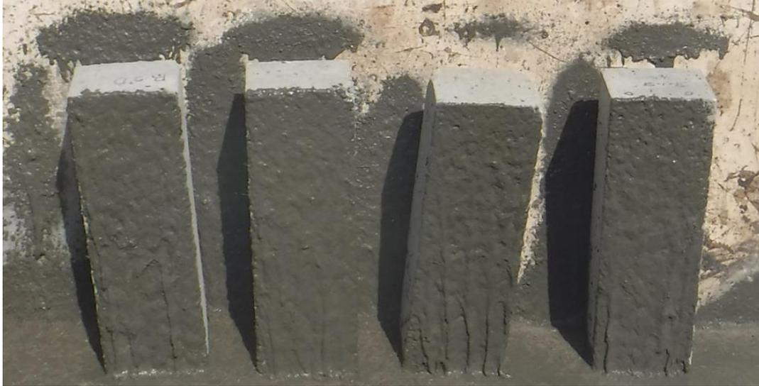
**Figure 15.** Horizontal application on flexural beam samples
