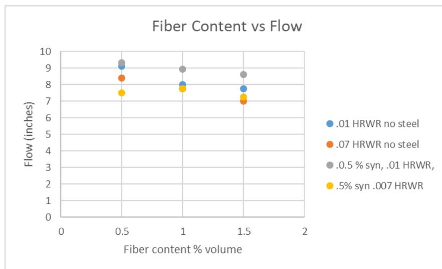
**Figure 6.** Fiber Content vs Flow.
