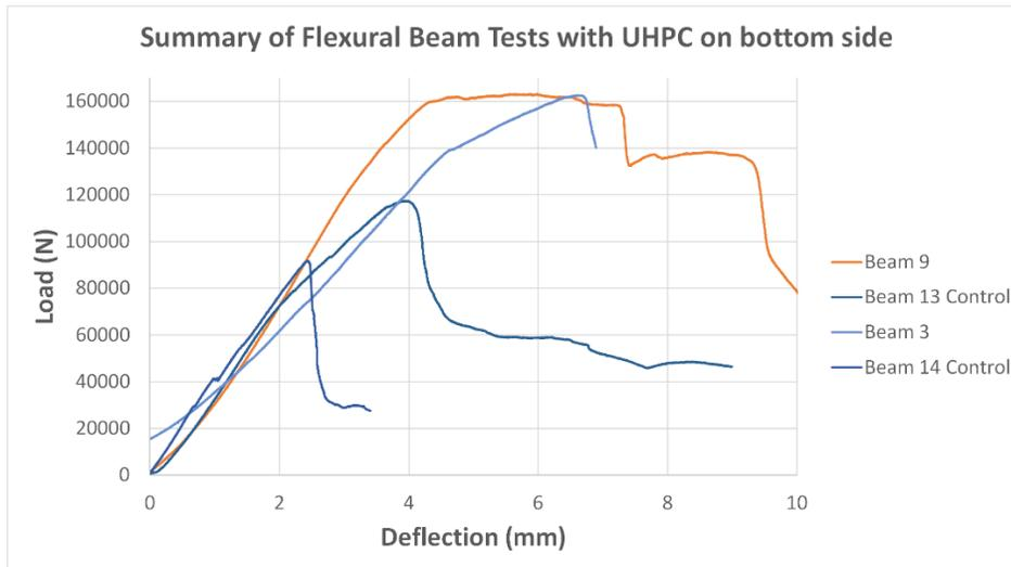
**Figure 19.** Summary of Flexural Beam tests with UHPC on Bottom side
