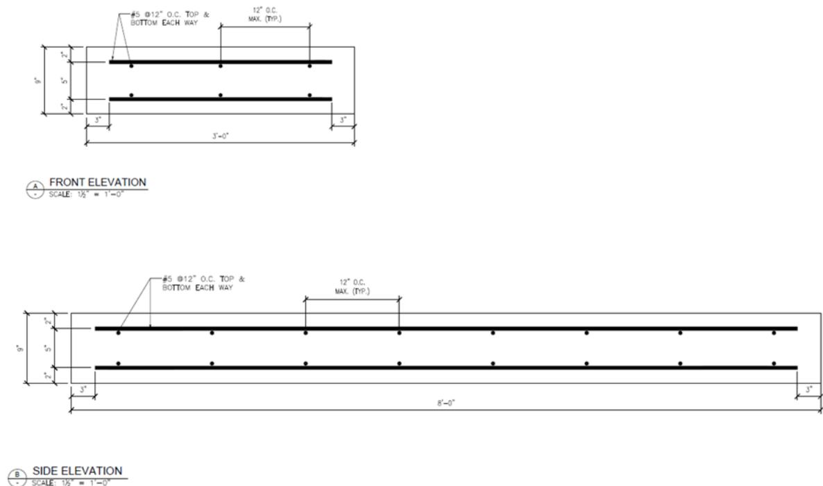
**Figure 10.** Details of the first specimen (Benchmark)
