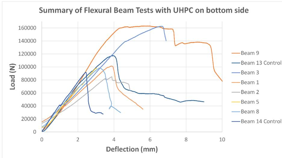
**Figure 17.** Summary of Flexural Beam tests with UHPC on Bottom side
