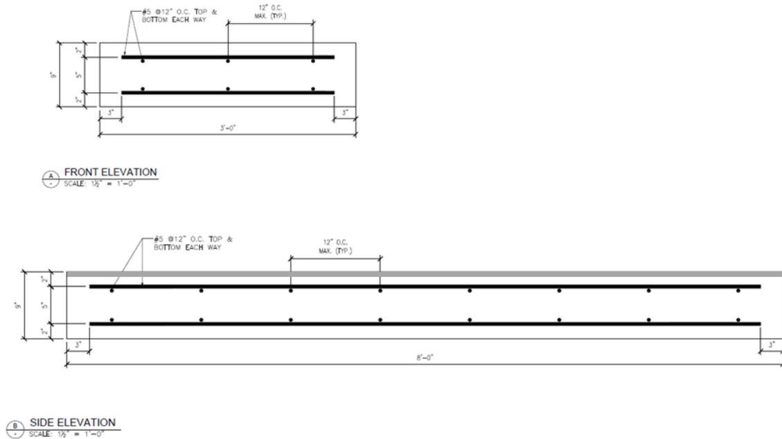
**Figure 12.** Details of the second specimen (Bridge Overlay)
