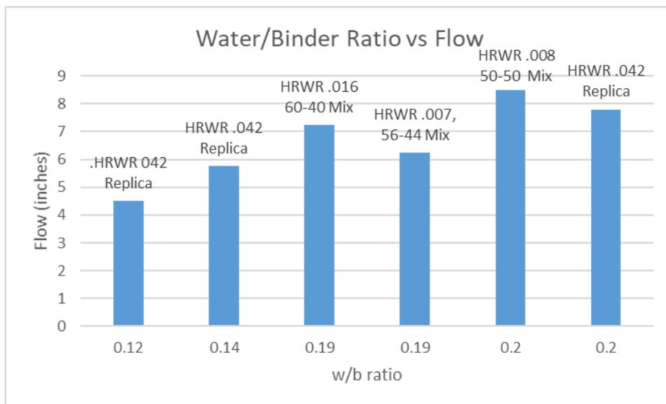
**Figure 8.** Water to Binder Ratio vs Flow.
