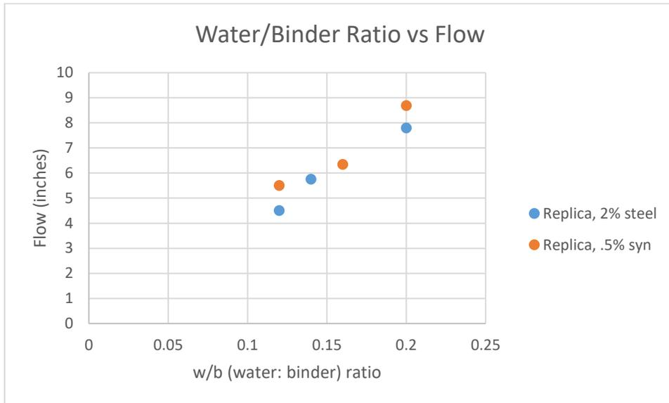
**Figure 7.** Water to Binder Ratio vs Flow, 57:43 Mix.
