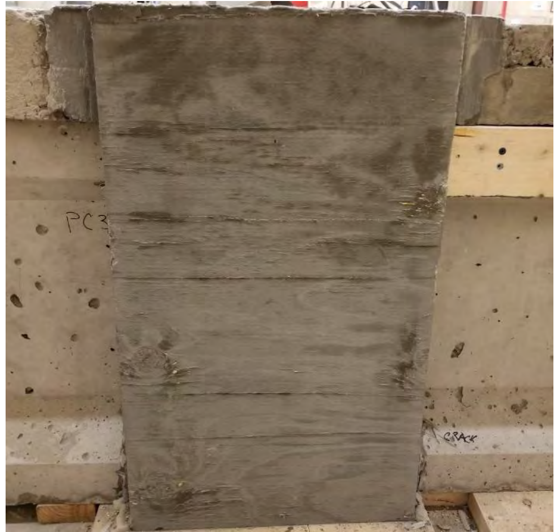
Retrofit construction continuity joint
