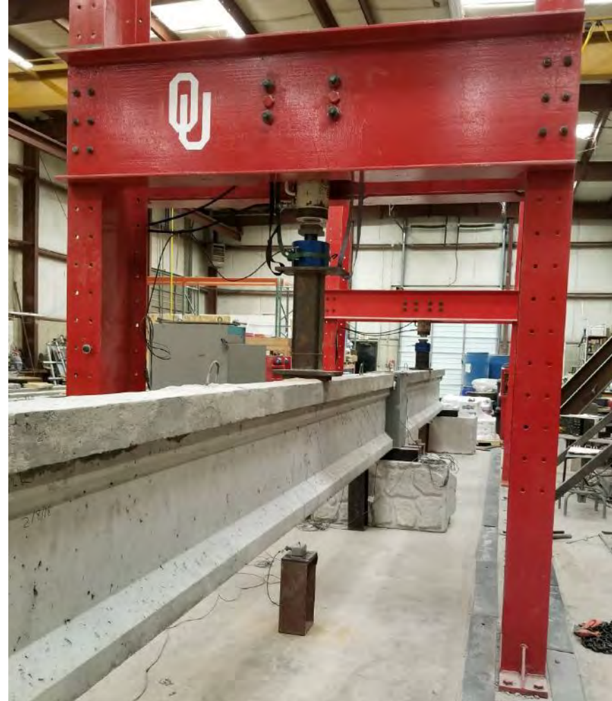
Two-span loading configuration used for testing continuity joints showing loads applied at mid-span of each beam
