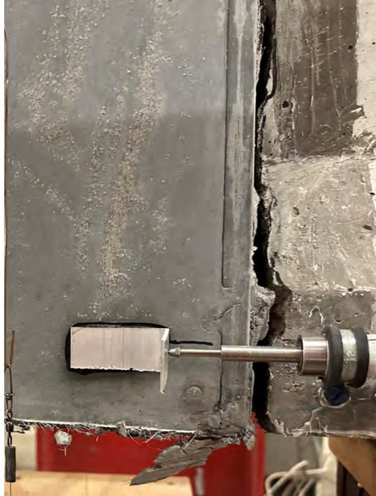
Typical separation at the interface between the girder and UHPC connection
