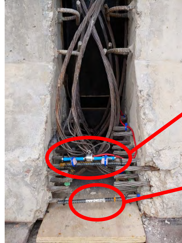
Instrumentation for UHPC joint
