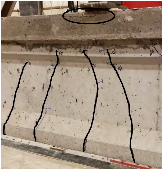
Flexural cracking under load point
