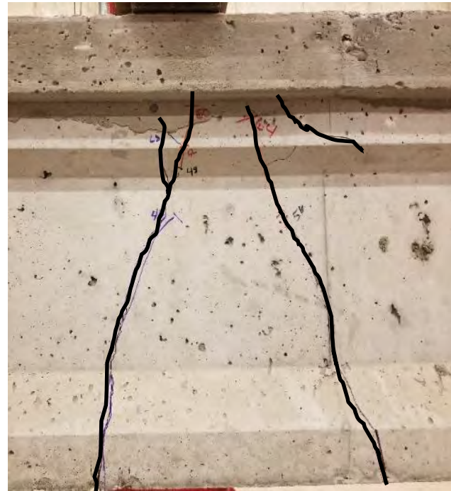
Flexural cracking under load point
