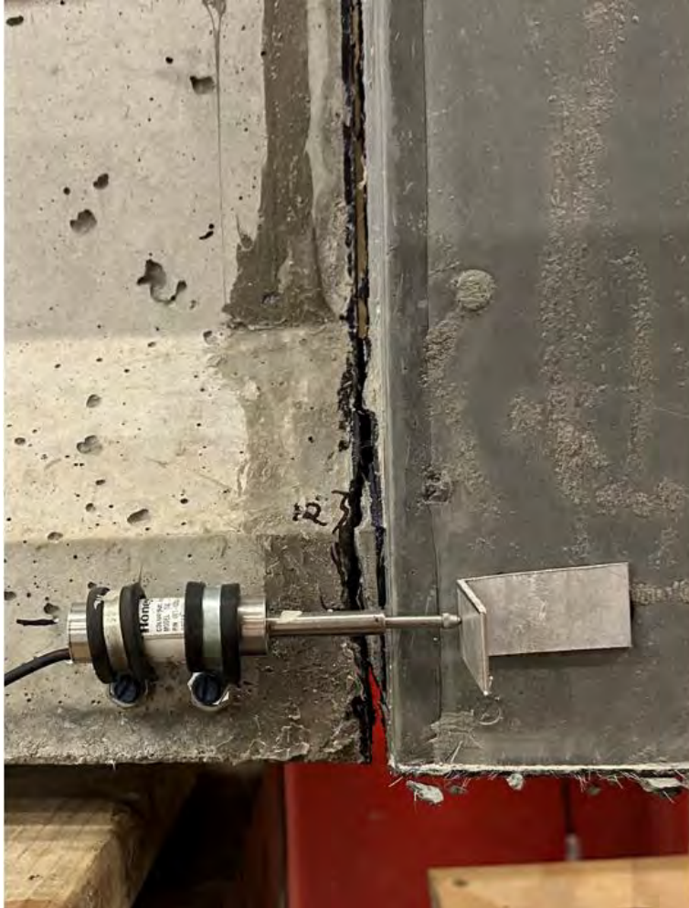
Typical separation at the interface between the girder and UHPC connection
