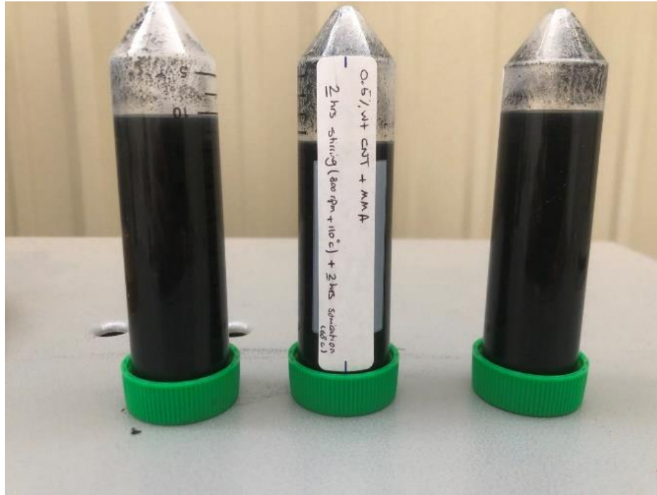
Figure 13 Uniform composite after dispersion (0.5 wt.% COOH in MMA resin)
