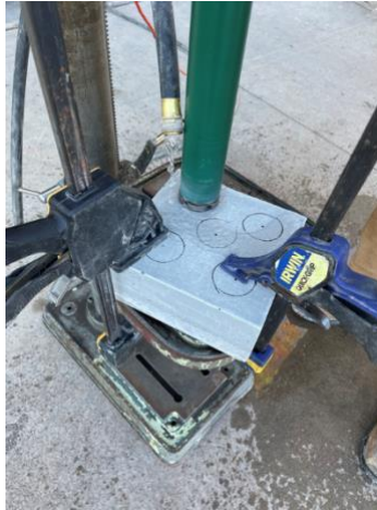
Figure 9 Core drilling using universal drilling machine
