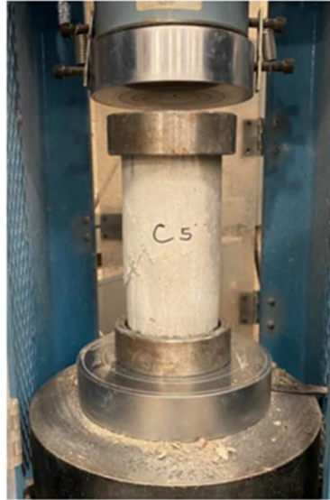
Figure 4 Compression Test Result of PolC Failed Specimen
