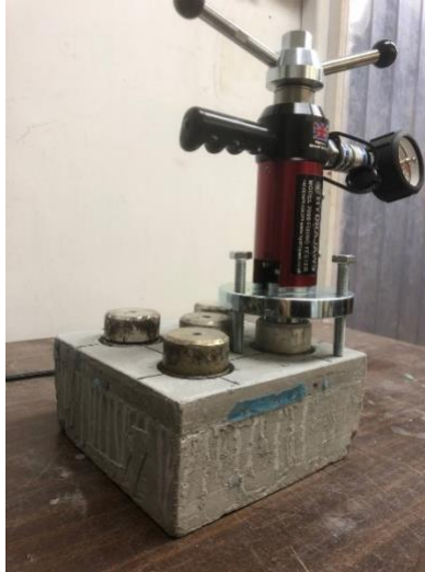
Figure 10 Pull off tests on cores
