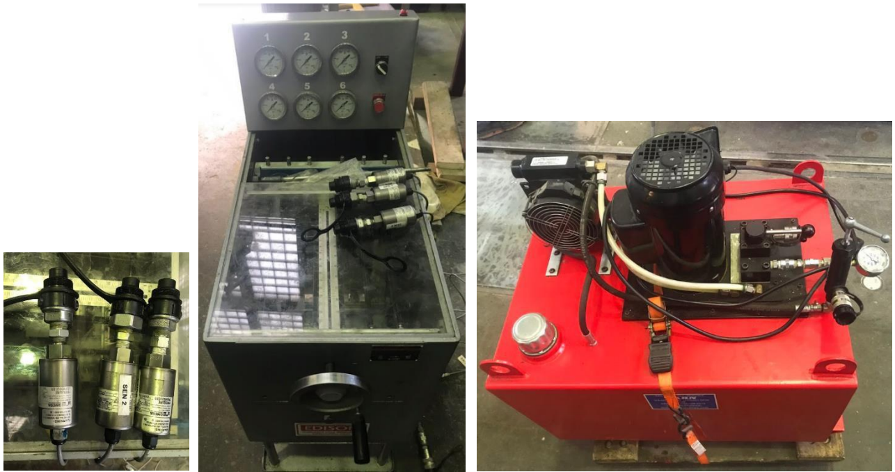
Figure A.5: Panel test equipment (a) pressure sensors, (b) load maintainer, and (c) hydraulic pump
