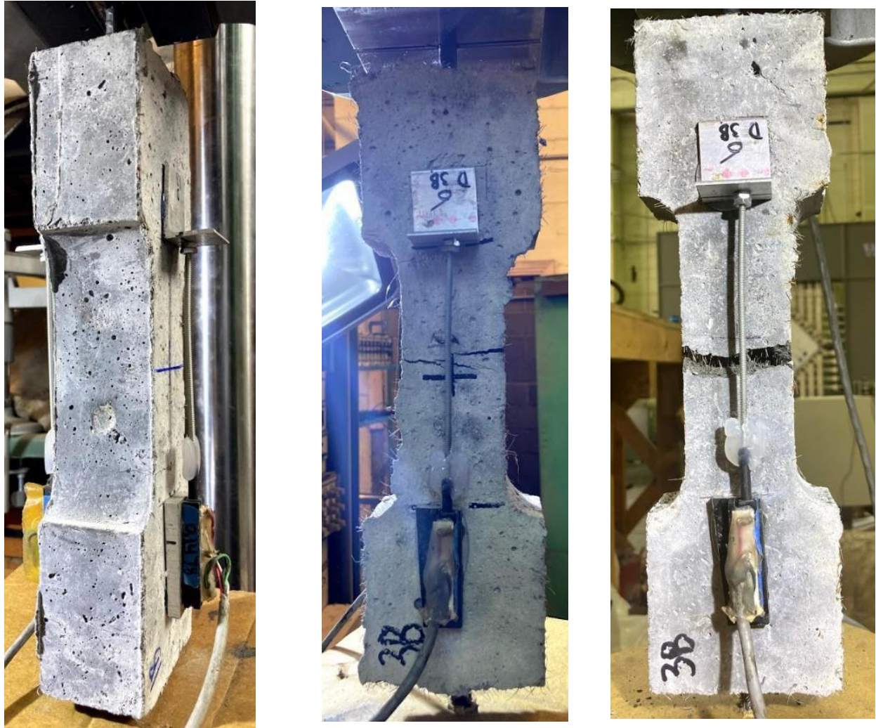
Figure A.3: Direct tension test (a) setup, (b) typical cracking, (c) typical failure
