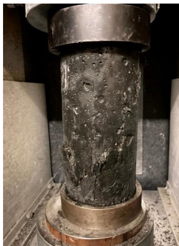
Figure 3.1: Typical compression failure
