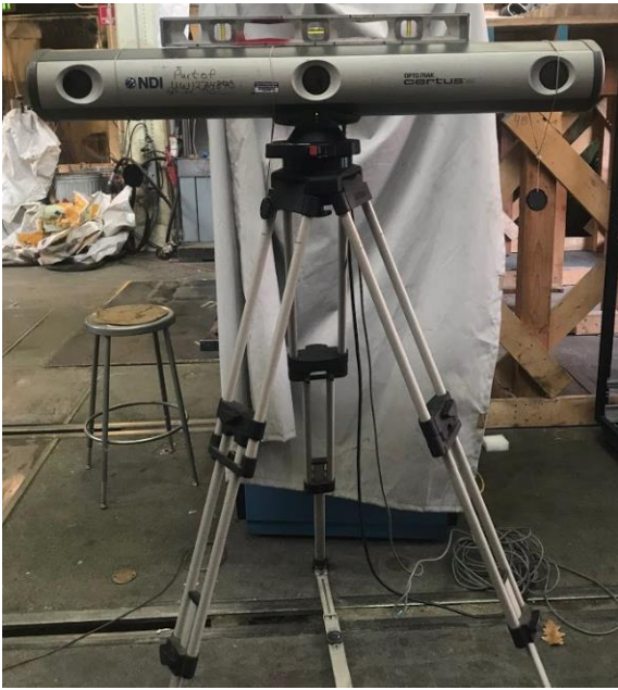
Figure 3.11: (a) Optotrak targets (b) Optotrak camera (c) test setup
