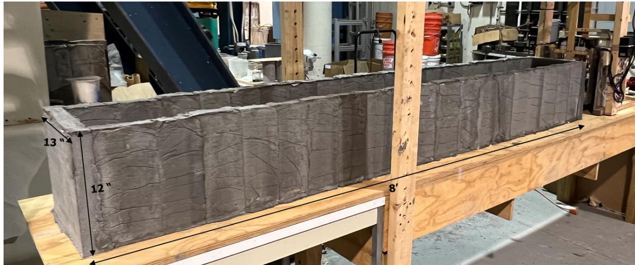
Figure 9: 3D printed beam section
