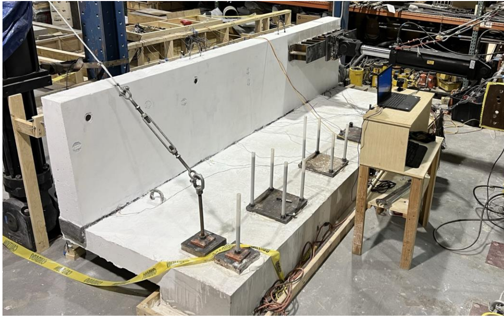
Figure 18- Test setup for the full-scale 15 ft long barrier specimen with UHPC connection.
