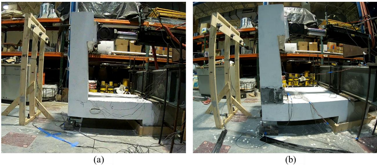
Figure 9- Load test setup for a) cast-in-place barrier and b) prefabricated barrier with UHPC connection.
