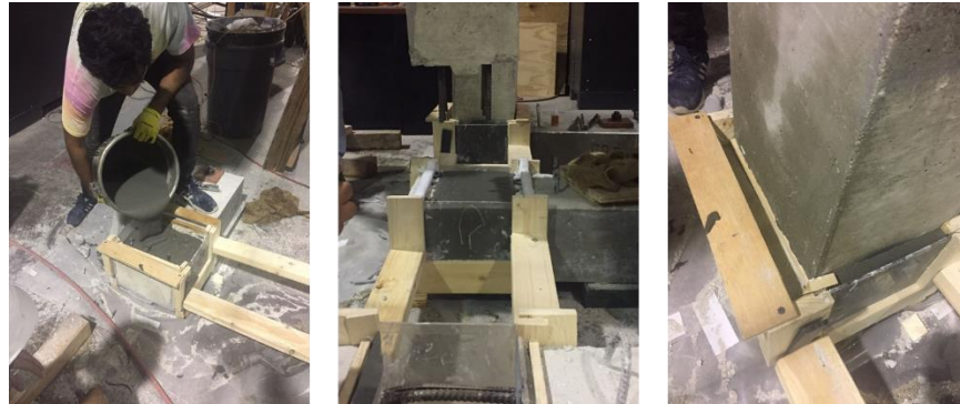
Figure 12- Construction of Specimen 2 with shear key and dowels.
