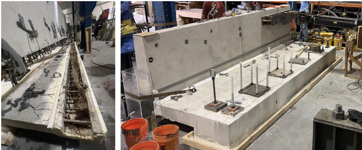
Figure 17- Construction of the full-scale 15 ft. long barrier specimen with UHPC connection.
