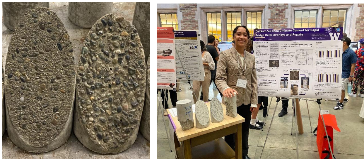
Fig. 1. Preliminary slant shear testing (a) achieved substrate surfaces (b) poster presentation
