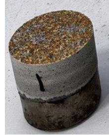
Failure in interface of concrete substrate-polymer concrete
