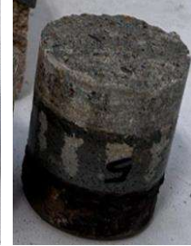
Failure in concrete substrate
