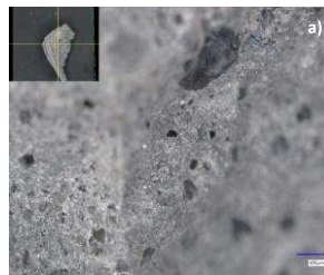
Fracture surface showing small dark particles spread across homogeneously
