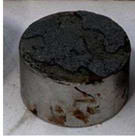
Failure in polymer concrete
