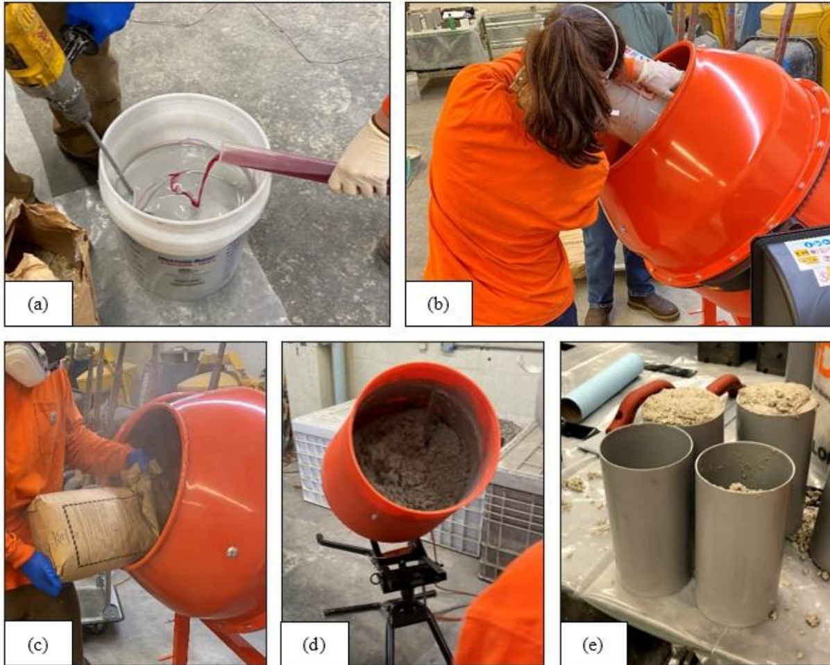
Figure 3-3. (a) Mixing of MEKP and HCSC resin with a squirrel cage mixer, (b) Resin mixture being transferred from mixing bucket to drum mixing, (c) Adding the pre-packaged aggregate and fiber blend to the drum mixer, (d) HCSC mix turning in drum mixer, (e) HCSC placed in cylinder molds before finishing
