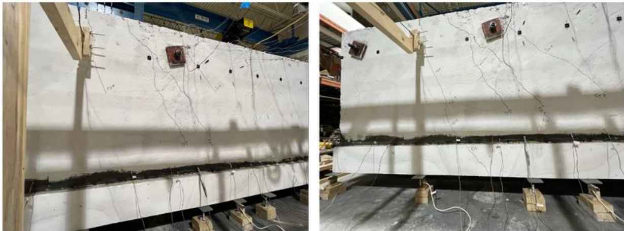
(c) Development of cracks at the backside of the barrier ( 57 \text{ kip} < P < 70 \text{ kip} )
