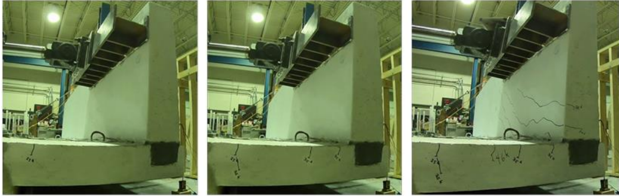
(a) Initial cracking in the deck overhang and the barrier ( P < 54 kip)
