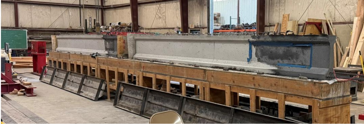
Figure 5. Completed hybrid girder specimens
