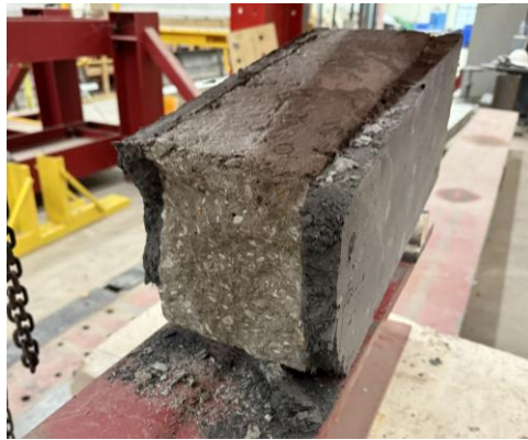
Figure 8. Fracture of UHPC shell specimen at failure
