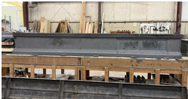
Figure 3. Completed UHPC prestressed girder specimen
