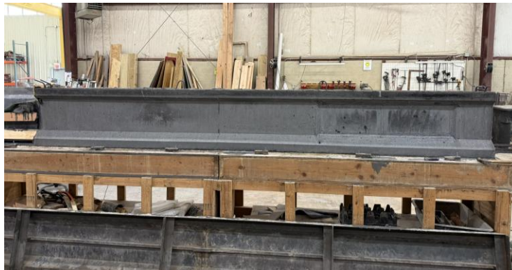
Figure 3. Completed UHPC prestressed girder specimen
