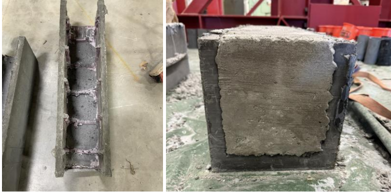
Figure 7. UHPC shell (left) and completed modulus of rupture specimen (right)
