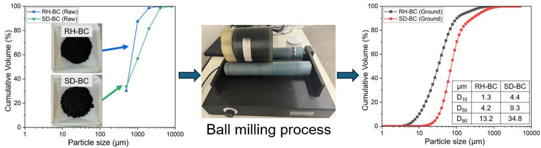
Figure 2.1 Biochar ball milling procedure, showing the as-received particle size distribution (left) and the ground size distribution after milling (right).
