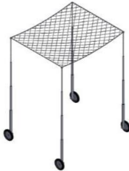
Figure 4: Basic Design of Proposed Net (created in SolidWorks)
