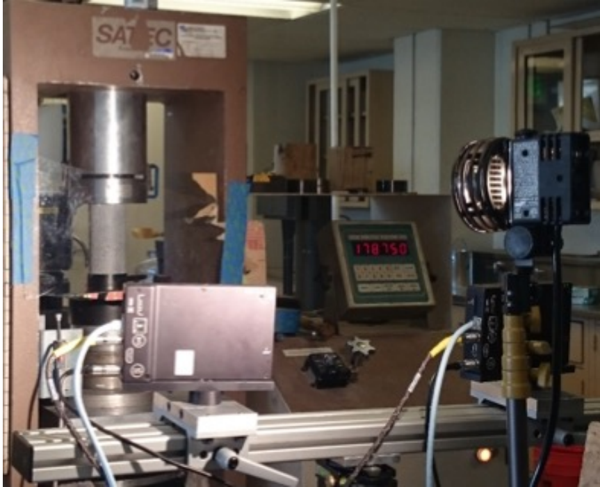
Figure 8. UHPC compression test set-up.
