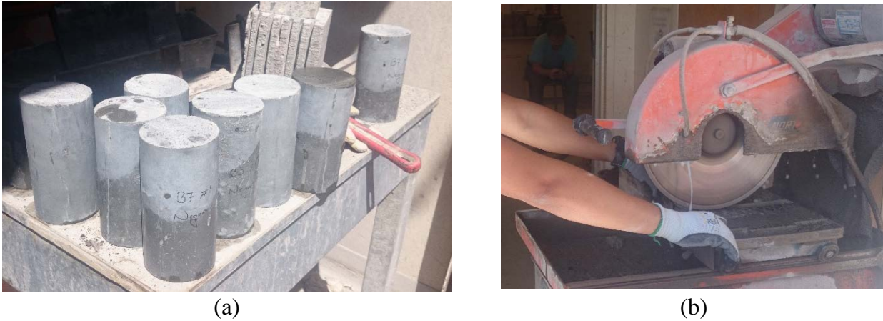
Figure 5. (a) Demolded UHPC Cylinders (b) Saw cutting of cylinders.
