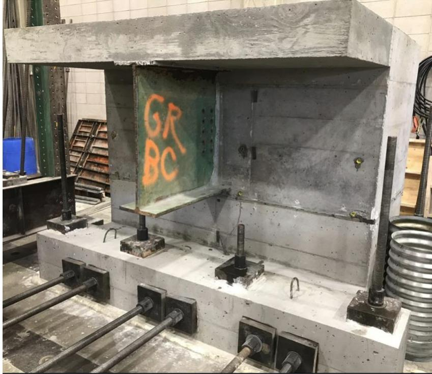
**Figure 2.** Grouted Reinforcing Bar Coupler connection completed.
