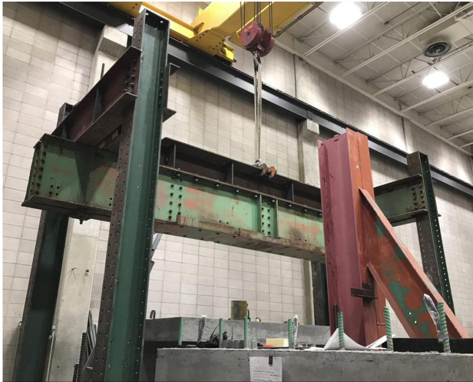
**Figure 3.** Grouted Reinforcing Bar Coupler Loading Setup.
