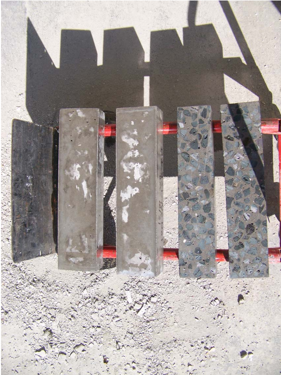
Photo 1 – Saw Cut Faces of Beams
