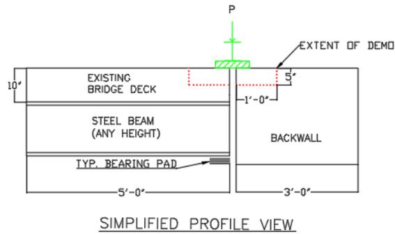
2. End rotation will be measured during all tests
