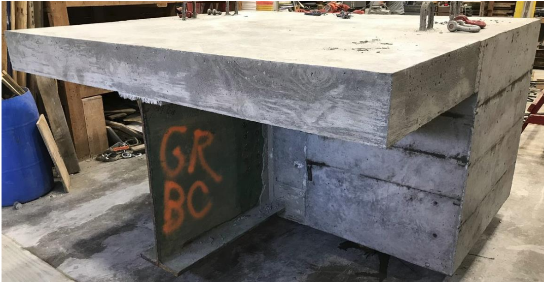
Figure 2. Grouted Reinforcing Bar Coupler Integral Diaphragm completed.
