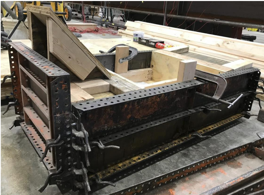
Figure 3. Flowability test formwork.
