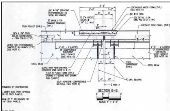
Fig.11: UHPC Link Slab Design
