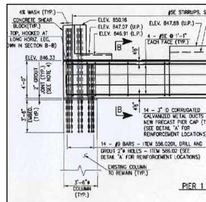
Fig.5: Originally Specified Pier Cap Connection
