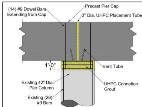
Fig.7: UHPC Placement (10)
