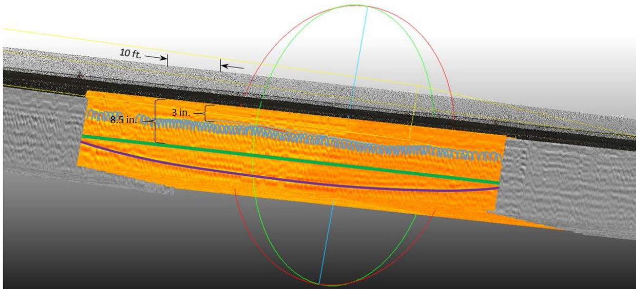
Figure 1. Keg Creek Bridge results showing fused GPR and LIDAR results in a zoom view of span 2 plus reinforcing steel (light blue hyperbolas), concrete deck bottom surface reflection (green), and steel beam (purple) responses
