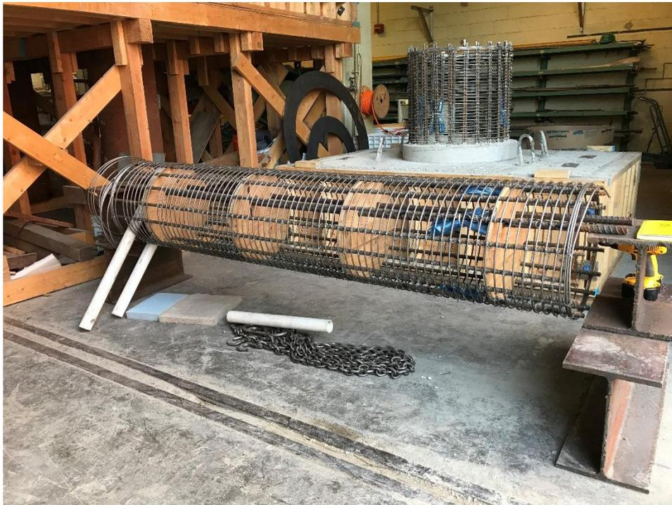
*Figure 4. Photo of Column Reinforcement Cage*
