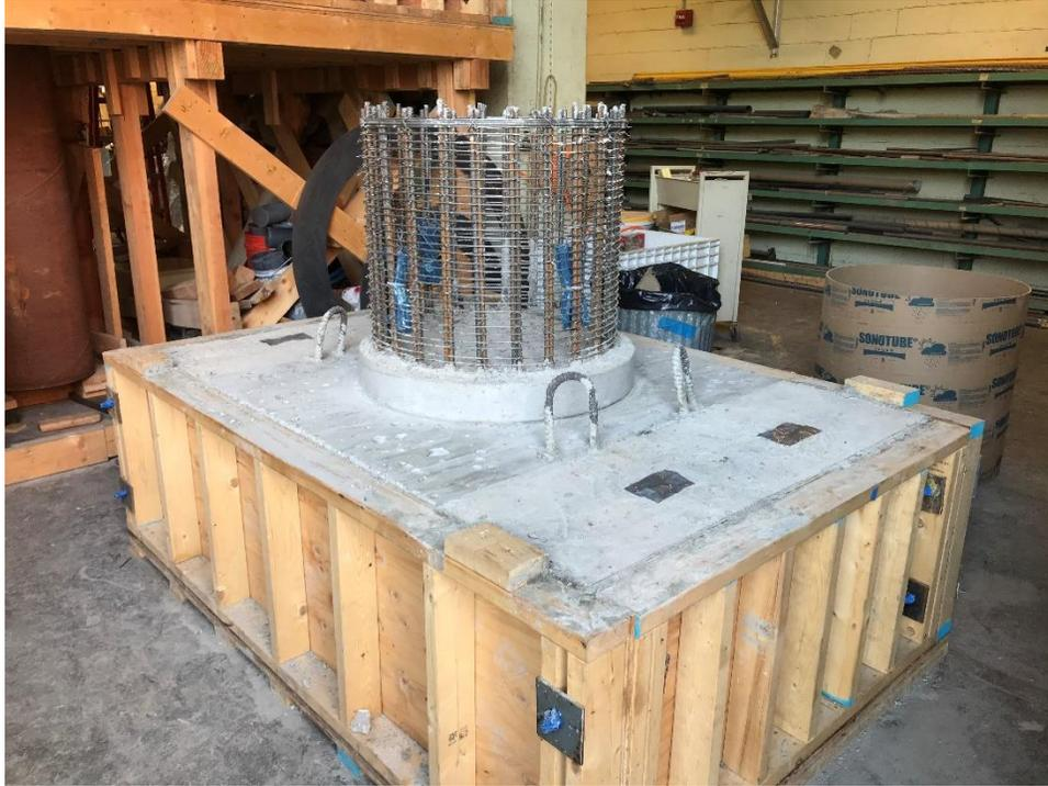
*Figure 3. Photo of Shaft Reinforcement and Cast Base*
