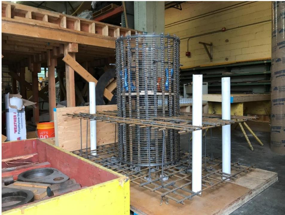
*Figure 2. Photo of Shaft and Base Reinforcement*
