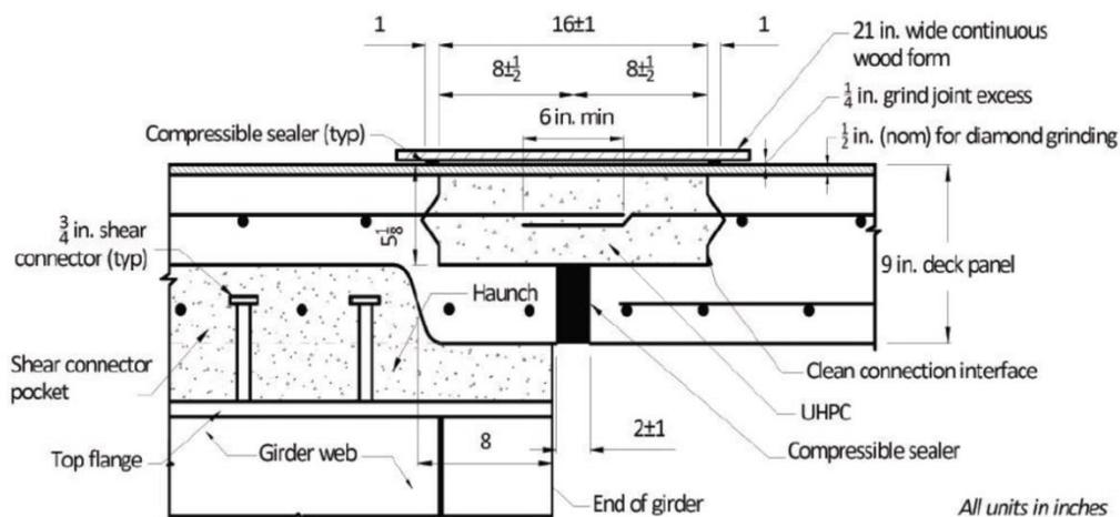
Figure 1. Example UHPC link slab detail used on a bridge project in Owego, NY, shown as a split section with the left side showing details at the girder line and right side showing details midway between girders (Graybeal, 2014)
