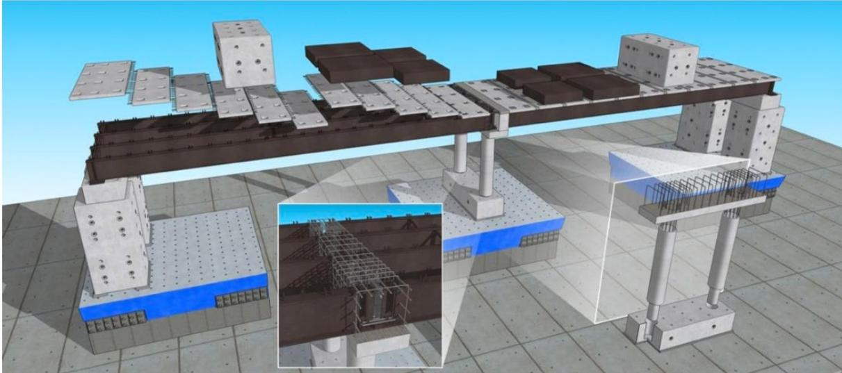
Figure 1: Three-dimensional view of the tested bridge model (Shoushtari et al. 2019).
