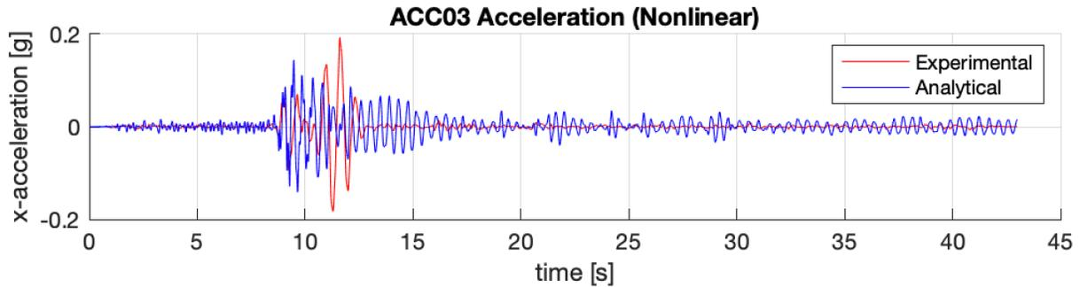
Figure 4: Comparison of numerically computed and experimental acceleration data in x-direction at ACC03 (Figure 3).
