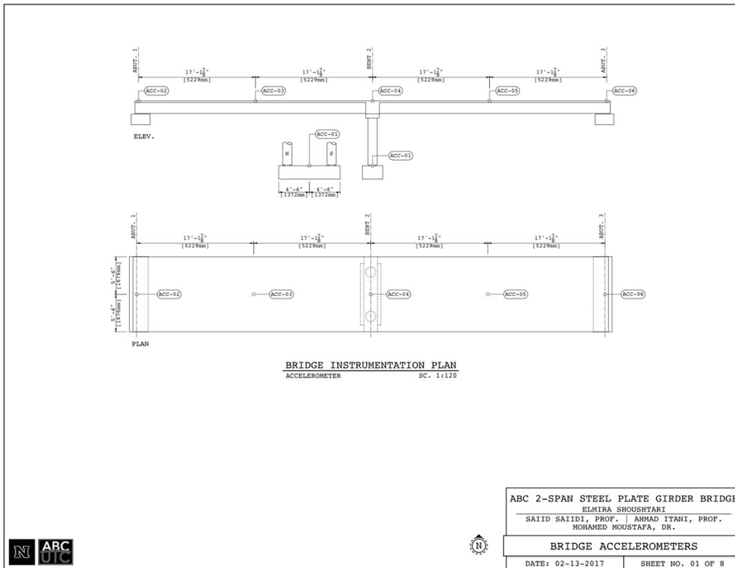
Figure 3: Locations of installed accelerometers.
