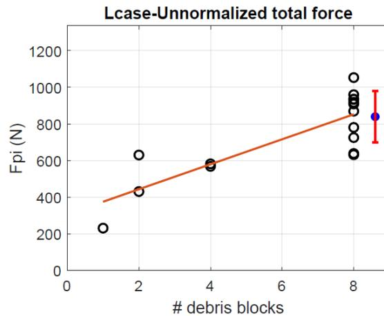
Figure 3. Effects of # Debris on Measured Peak Force
